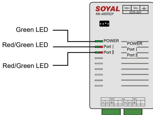
1. Green LED (Power) will keep lighting up when powering on.
